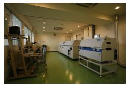
In our demo room, we use the circuit boards, components, and other workpieces that our customers use to create the optimal temperature profile on the actual machine (demo machine). We also provide peripheral equipment such as microscopes so that you can actually check the finish and quality of the product.
